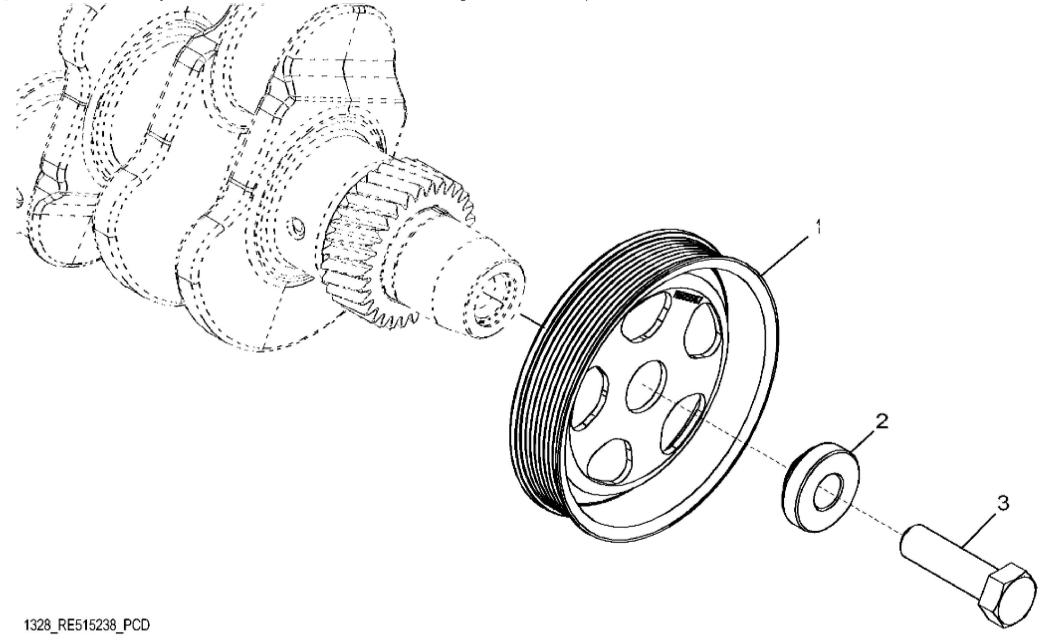
John Deere > Turf And Utility >TRACTOR >5100GF - TRACTOR >5100GF Tractor (Engine 4045HAT82)(Europe Edition) >24 ENGINE 4045HAT82-DD21694 >ST628039 - 1328 CRANKSHAFT PULLEY
