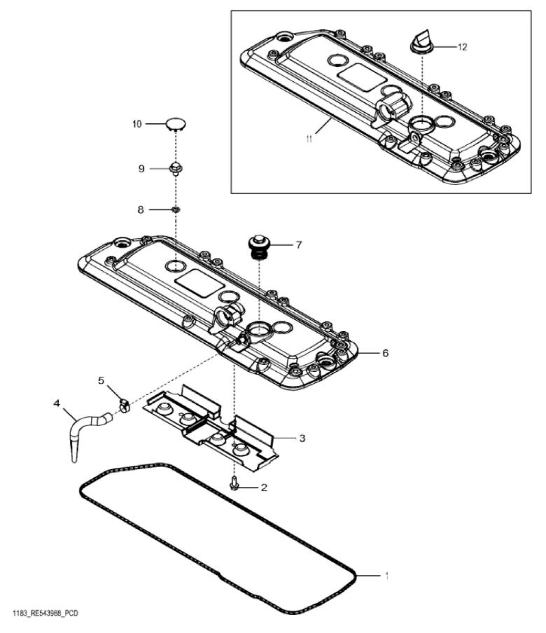
John Deere > Turf And Utility >TRACTOR >6115R - TRACTOR >6115R Tractor (Europe Edition, Engine SN: 4045RXXXXX)(Interim Tier 4) >20 ENGINE 4045HL495-DD22036-ETN65520-ETN65518-ETN74307 >ST400926 - 1183 ROCKER ARM COVER
