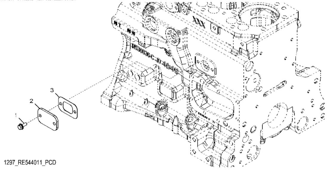
John Deere > Turf And Utility >TRACTOR >6115R - TRACTOR >6115R Tractor (Europe Edition, Engine SN: 4045RXXXXX)(Interim Tier 4) >20 ENGINE 4045HL495-DD22036-ETN65520-ETN65518-ETN74307 >ST402282 - 1297 OIL FILLER COVER
