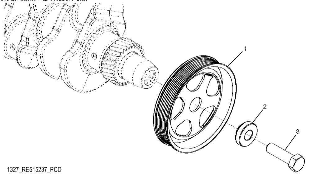
John Deere > Turf And Utility >TRACTOR >6115R - TRACTOR >6115R Tractor (Europe Edition, Engine SN: 4045RXXXXX)(Interim Tier 4) >20 ENGINE 4045HL495-DD22036-ETN65520-ETN65518-ETN74307 >ST308624 - 1327 CRANKSHAFT PULLEY
