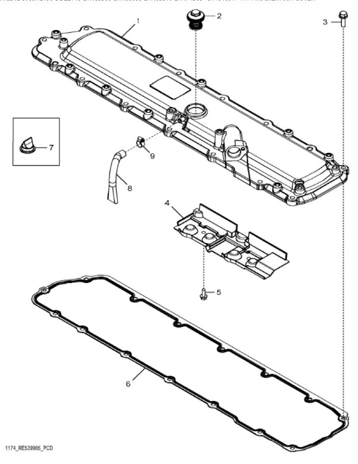
John Deere > Turf And Utility >TRACTOR >6140R - TRACTOR >6140R Tractor (Europe Edition, Engine SN: 4045RXXXXXX)(Interim Tier 4) >20 ENGINE 6068HL490-DD22146-ETN65508-ETN68088-ETN65510-ETN74309 >ST164694 - 1174 ROCKER ARM COVER
