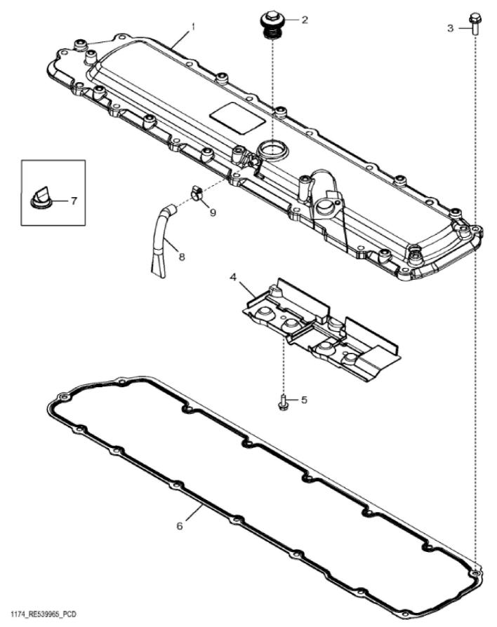
John Deere > Turf And Utility >TRACTOR >6150R - TRACTOR >6150R, 6150RH Tractor (North America Edition, Engine SN: 6068RXXXXXX)(Interim Tier 4) >20 ENGINE 6068RW405-RE549557-ETN90011-ETN90010 >ST164694 - 1174 ROCKER ARM COVER
