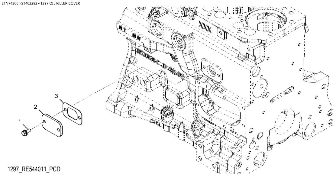
John Deere > Turf And Utility >TRACTOR >6115M - TRACTOR >6115M Tractor (Europe Edition, Engine SN: 4045RXXXXXX)(Interim Tier 4) >20 ENGINE 4045HL497-DD22038-ETN65521-ETN65522-ETN74306 >ST402282 - 1297 OIL FILLER COVER
