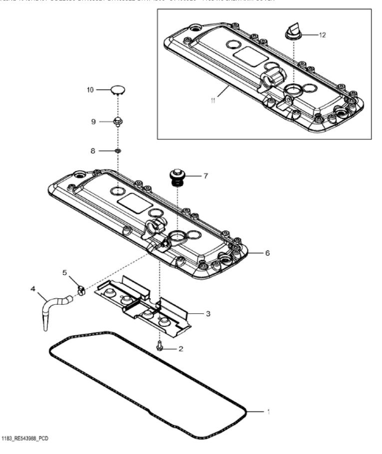
John Deere > Turf And Utility >TRACTOR >6115M - TRACTOR >6115M Tractor (Europe Edition, Engine SN: 4045RXXXXXX)(Interim Tier 4) >20 ENGINE 4045HL497-DD22038-ETN65521-ETN65522-ETN74306 >ST400926 - 1183 ROCKER ARM COVER
