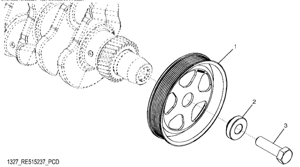
John Deere > Turf And Utility >TRACTOR >6130M - TRACTOR >6130M Tractor (Europe Edition, Engine SN: 4045RXXXXX)(Interim Tier 4) >20 ENGINE 4045HL496-DD22037-ETN65516-ETN65517-ETN74308 >ST308624 - 1327 CRANKSHAFT PULLEY
