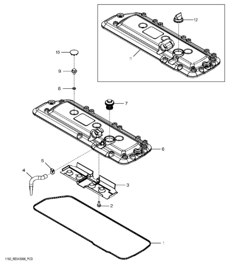
John Deere > Turf And Utility >TRACTOR >6130M - TRACTOR >6130M Tractor (Europe Edition, Engine SN: 4045RXXXXX)(Interim Tier 4) >20 ENGINE 4045HL496-DD22037-ETN65516-ETN65517-ETN74308 >ST400926 - 1183 ROCKER ARM COVER
