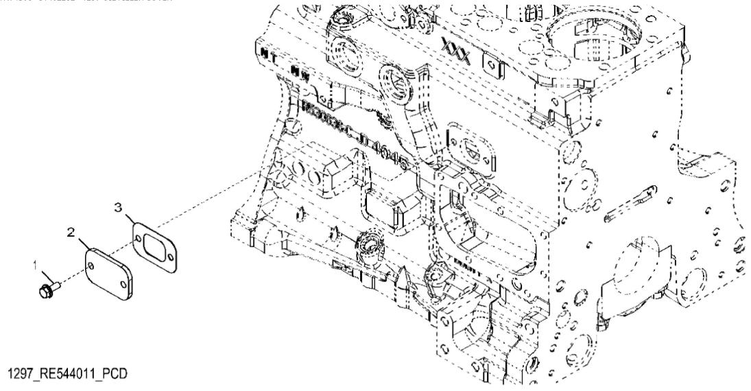
John Deere > Turf And Utility >TRACTOR >6130M - TRACTOR >6130M Tractor (Europe Edition, Engine SN: 4045RXXXXX)(Interim Tier 4) >20 ENGINE 4045HL496-DD22037-ETN65516-ETN65517-ETN74308 >ST402282 - 1297 OIL FILLER COVER
