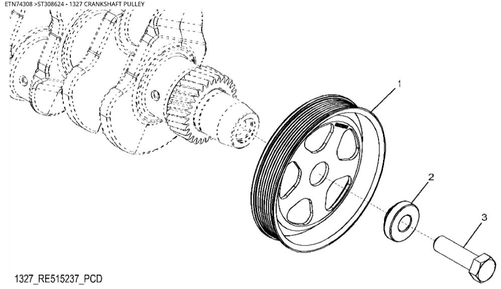
John Deere > Turf And Utility >TRACTOR >6140M - TRACTOR >6140M Tractor (Europe Edition, Engine SN: 4045RXXXXXX)(Interim Tier 4) >20 ENGINE 4045HL496-DD22037-ETN65516-ETN65517-ETN74308 >ST308624 - 1327 CRANKSHAFT PULLEY
