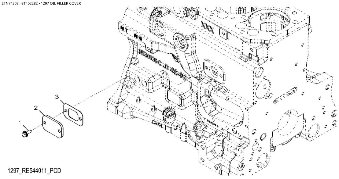
John Deere > Turf And Utility >TRACTOR >6140M - TRACTOR >6140M Tractor (Europe Edition, Engine SN: 4045RXXXXXX)(Interim Tier 4) >20 ENGINE 4045HL496-DD22037-ETN65516-ETN65517-ETN74308 >ST402282 - 1297 OIL FILLER COVER
