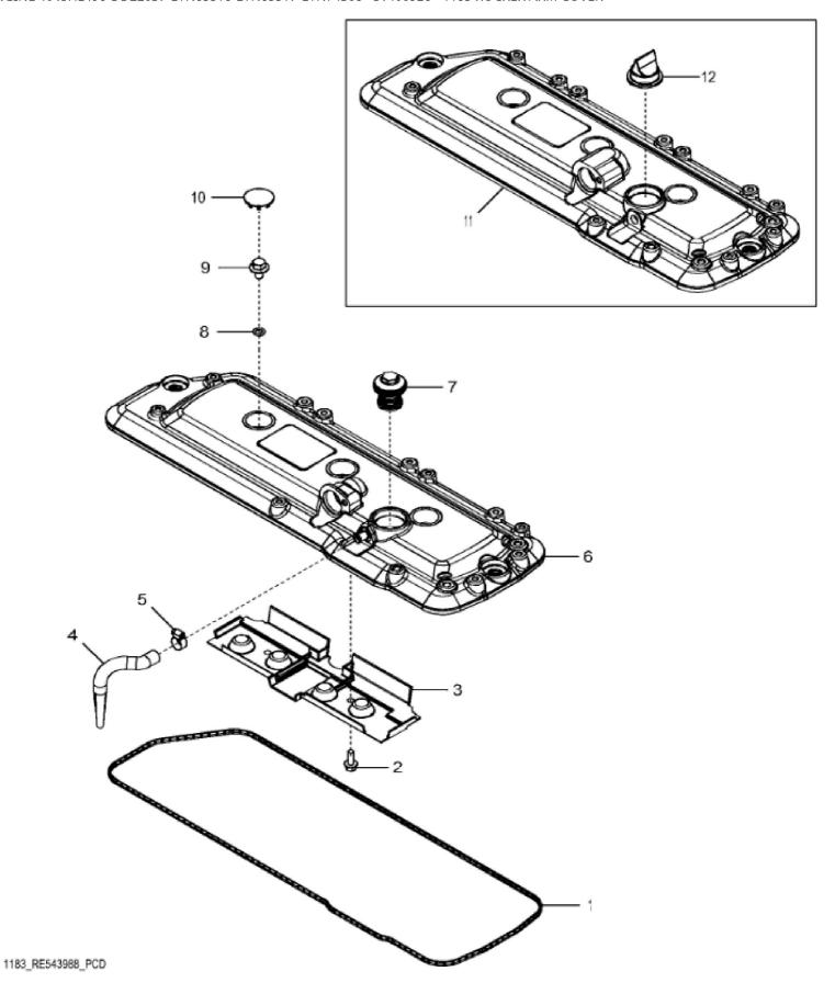
John Deere > Turf And Utility >TRACTOR >6140M - TRACTOR >6140M Tractor (Europe Edition, Engine SN: 4045RXXXXXX)(Interim Tier 4) >20 ENGINE 4045HL496-DD22037-ETN65516-ETN65517-ETN74308 >ST400926 - 1183 ROCKER ARM COVER
