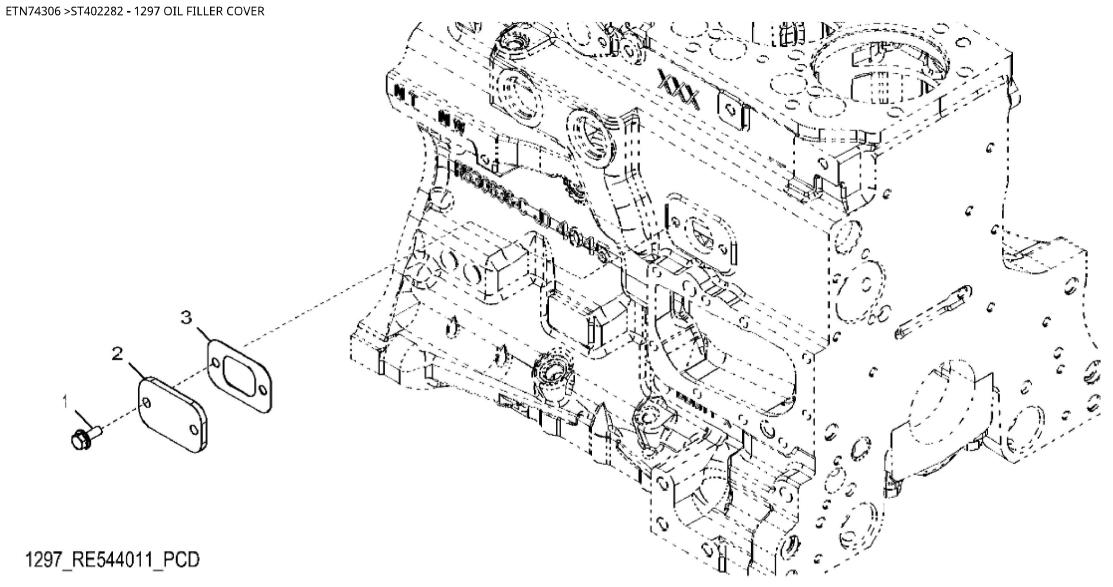
John Deere > Turf And Utility >TRACTOR >6115M - TRACTOR >6115M Tractor (North America Edition, Engine SN: 4045RXXXXXX)(Interim Tier 4) >20 ENGINE 4045HL497-DD22038-ETN65521-ETN65522-ETN74306 >ST402282 - 1297 OIL FILLER COVER
