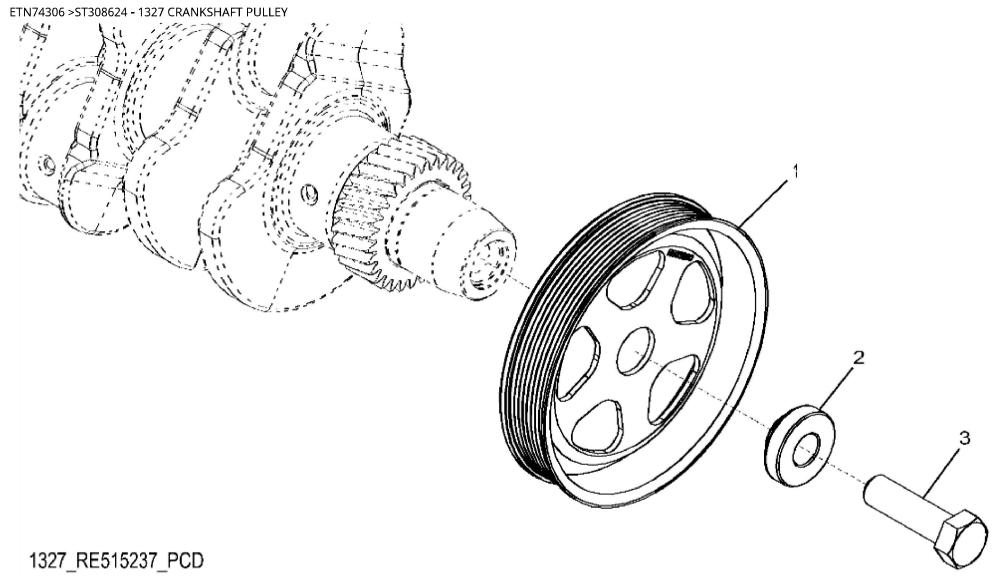
John Deere > Turf And Utility >TRACTOR >6115M - TRACTOR >6115M Tractor (North America Edition, Engine SN: 4045RXXXXXX)(Interim Tier 4) >20 ENGINE 4045HL497-DD22038-ETN65521-ETN65522-ETN74306 >ST308624 - 1327 CRANKSHAFT PULLEY
