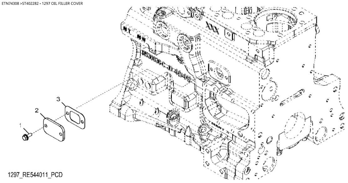
John Deere > Turf And Utility >TRACTOR >6140M - TRACTOR >6140M Tractor (North America Edition, Engine SN: 4045RXXXXXX)(Interim Tier 4) >20 ENGINE 4045HL496-DD22037-ETN65516-ETN65517-ETN74308 >ST402282 - 1297 OIL FILLER COVER
