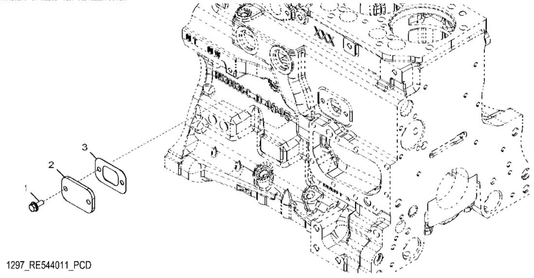
John Deere > Turf And Utility >TRACTOR >6110RC - TRACTOR >6110RC Tractor (Europe Edition, Engine SN: 4045RXXXXX)(Interim Tier 4) >20 ENGINE 4045HL490-DD22206-DD22370-ETN98548-ETN120276 >ST402282 - 1297 OIL FILLER COVER
