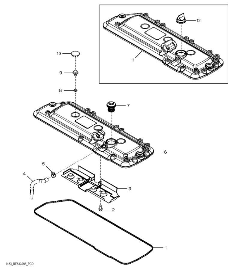
John Deere > Turf And Utility >TRACTOR >6110RC - TRACTOR >6110RC Tractor (Europe Edition, Engine SN: 4045RXXXXX)(Interim Tier 4) >20 ENGINE 4045HL490-DD22206-DD22370-ETN98548-ETN120276 >ST400926 - 1183 ROCKER ARM COVER
