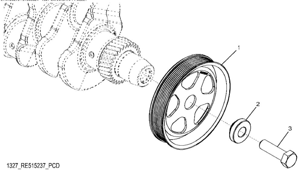
John Deere > Turf And Utility >TRACTOR >6110RC - TRACTOR >6110RC Tractor (Europe Edition, Engine SN: 4045RXXXXX)(Interim Tier 4) >20 ENGINE 4045HL490-DD22206-DD22370-ETN98548-ETN120276 >ST308624 - 1327 CRANKSHAFT PULLEY
