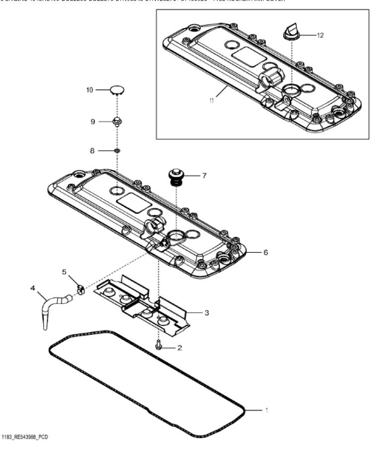
John Deere > Turf And Utility >TRACTOR >6090MC - TRACTOR >6090MC Tractor (Europe Edition, Engine SN: 4045RXXXXXX)(Interim Tier 4) >20 ENGINE 4045HL490-DD22206-DD22370-ETN98548-ETN120276 >ST400926 - 1183 ROCKER ARM COVER
