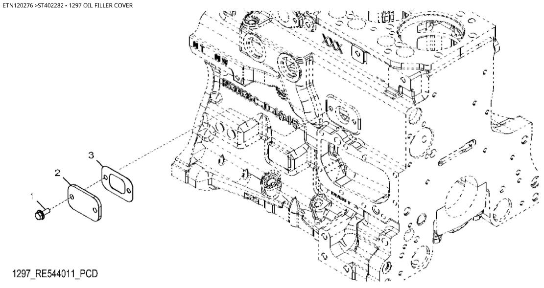
John Deere > Turf And Utility >TRACTOR >6090MC - TRACTOR >6090MC Tractor (Europe Edition, Engine SN: 4045RXXXXXX)(Interim Tier 4) >20 ENGINE 4045HL490-DD22206-DD22370-ETN98548-ETN120276 >ST402282 - 1297 OIL FILLER COVER
