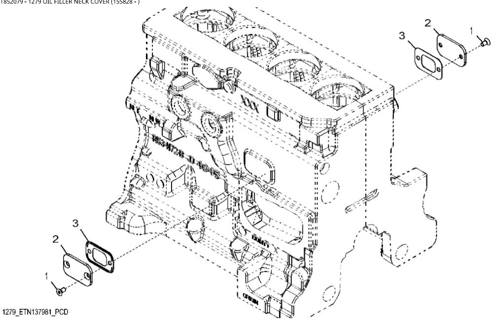
John Deere > Turf And Utility >TRACTOR >6125M - TRACTOR >6125M Tractor (Europe Edition, Engine SN: 4045GXXXXXX)(Tier 2)(S.N. -859288) >20 ENGINE 4045HL289-DD22383-DD22435-ETN108061 >ST852079 - 1279 OIL FILLER NECK COVER (155828 - )
