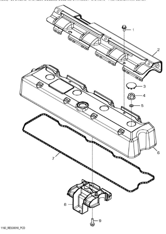
John Deere > Turf And Utility >TRACTOR >6125M - TRACTOR >6125M Tractor (Europe Edition, Engine SN: 4045GXXXXXX)(Tier 2)(S.N. -859288) >20 ENGINE 4045HL289-DD22383-DD22435-ETN108061 >ST349518 - 1160 ROCKER ARM COVER
