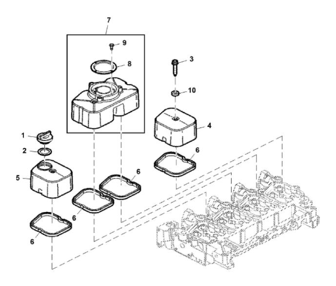
John Deere > Turf And Utility >TRACTOR >5100GN - TRACTOR >5100GN Tractor (Engine F4C) T3A (Europe Edition) >20 ENGINE >ST810003 - CYLINDER HEAD COVER
