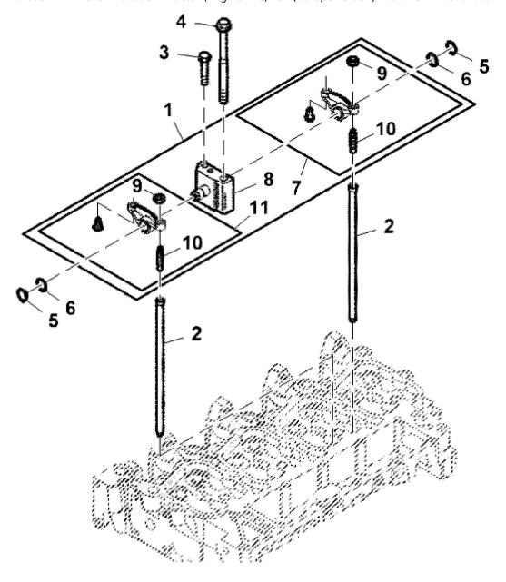
John Deere > Turf And Utility >TRACTOR >5100GN - TRACTOR >5100GN Tractor (Engine F4C) T3A (Europe Edition) >20 ENGINE >ST810081 - ROCKER ARM / SHAFT
