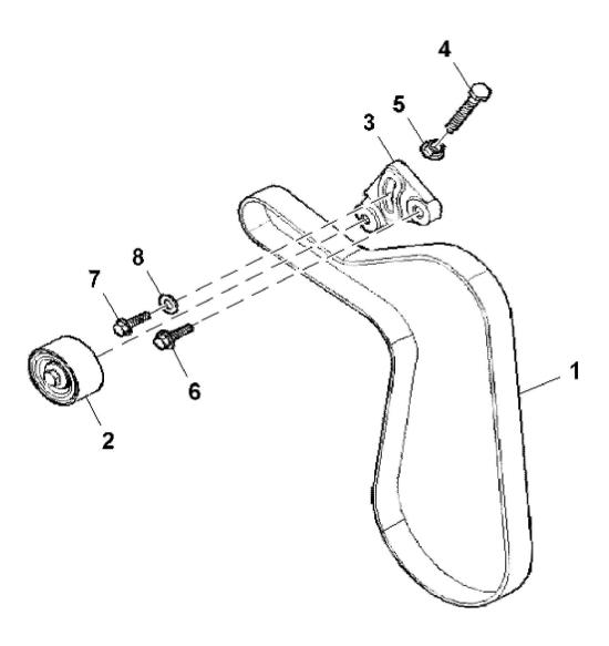
John Deere > Turf And Utility >TRACTOR >5100GN - TRACTOR >5100GN Tractor (Engine F4C) T3A (Europe Edition) >20 ENGINE >ST810175 - DRIVE BELT / PULLEY
