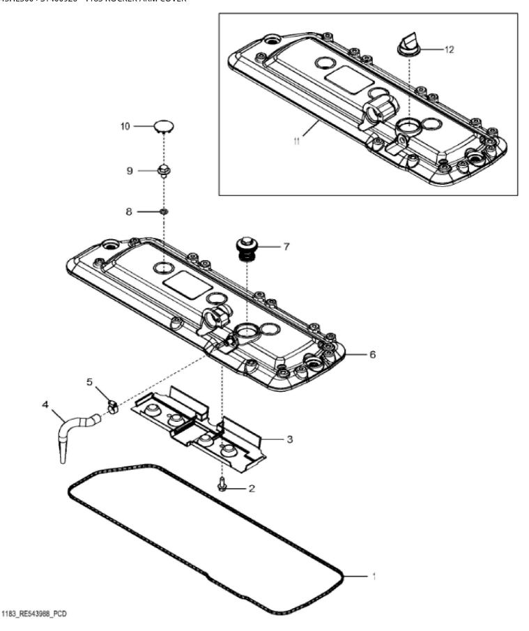
John Deere > Turf And Utility >TRACTOR >6120R - TRACTOR >6120R Tractor (Europe Edition, Engine SN: 4045UXXXXXX)(Final Tier 4) >E1 ENGINE 4045HL500-DD22292-ETN122284-ETN122286-ETN131686 >E100 ENGINE 4045HL500-DD22292-ETN122284-ETN122286-ETN131686 4045HL500 >ST400926 - 1183 ROCKER ARM COVER
