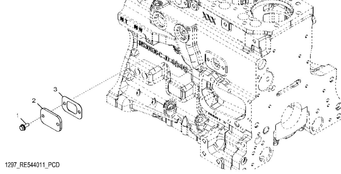
John Deere > Turf And Utility >TRACTOR >6130R - TRACTOR >6130R Tractor (Europe Edition, Engine SN: 4045UXXXXXX)(Final Tier 4) >E1 ENGINE 4045HL500-DD22292-ETN122284-ETN122286-ETN131686 >E100 ENGINE 4045HL500-DD22292-ETN122284-ETN122286-ETN131686 4045HL500 >ST402282 - 1297 OIL FILLER COVER
