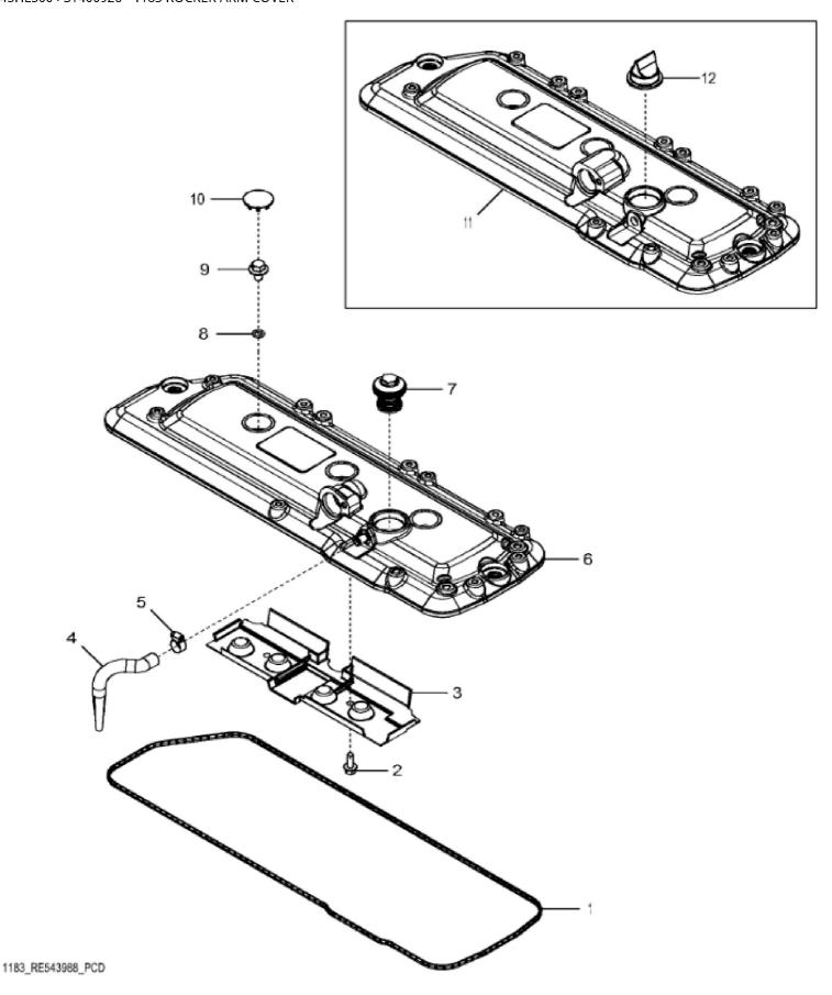
John Deere > Turf And Utility >TRACTOR >6130R - TRACTOR >6130R Tractor (Europe Edition, Engine SN: 4045UXXXXXX)(Final Tier 4) >E1 ENGINE 4045HL500-DD22292-ETN122284-ETN122286-ETN131686 >E100 ENGINE 4045HL500-DD22292-ETN122284-ETN122286-ETN131686 4045HL500 >ST400926 - 1183 ROCKER ARM COVER
