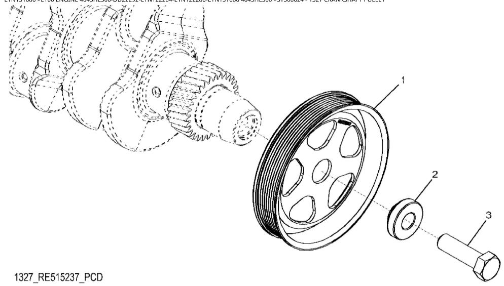
John Deere > Turf And Utility >TRACTOR >6130R - TRACTOR >6130R Tractor (Europe Edition, Engine SN: 4045UXXXXXX)(Final Tier 4) >E1 ENGINE 4045HL500-DD22292-ETN122284-ETN122286-ETN131686 >E100 ENGINE 4045HL500-DD22292-ETN122284-ETN122286-ETN131686 4045HL500 >ST308624 - 1327 CRANKSHAFT PULLEY
