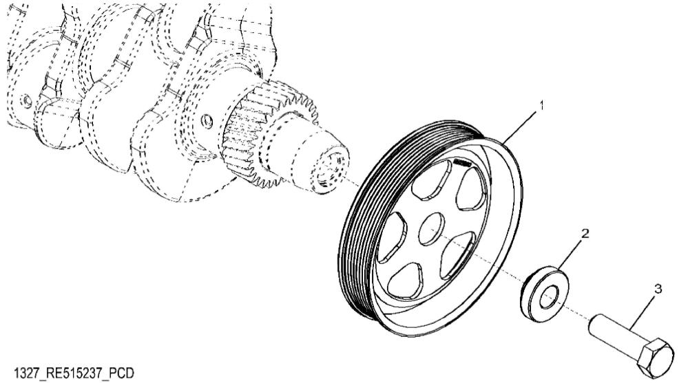
John Deere > Turf And Utility >TRACTOR >6135R - TRACTOR >6135R Tractor (Europe Edition, Engine SN: 4045UXXXXX)(Final Tier 4) >E1 ENGINE 4045HL501-DD22310-ETN124754-ETN131687 +1327 CRANKSHAFT PULLEY
