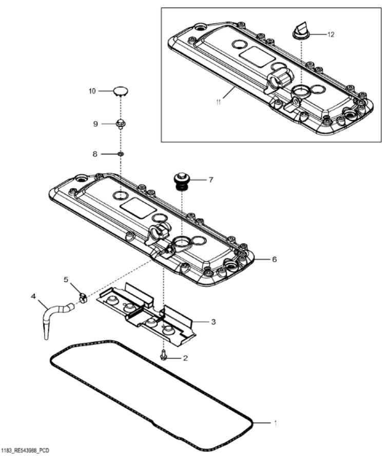
John Deere > Turf And Utility >TRACTOR >6135R - TRACTOR >6135R Tractor (Europe Edition, Engine SN: 4045UXXXXXX)(Final Tier 4) >E1 ENGINE 4045HL501-DD22310-ETN124754-ETN131687 >E100 ENGINE 4045HL501-DD22310-ETN124754-ETN131687 4045HL501 >ST400926 - 1183 ROCKER ARM COVER
