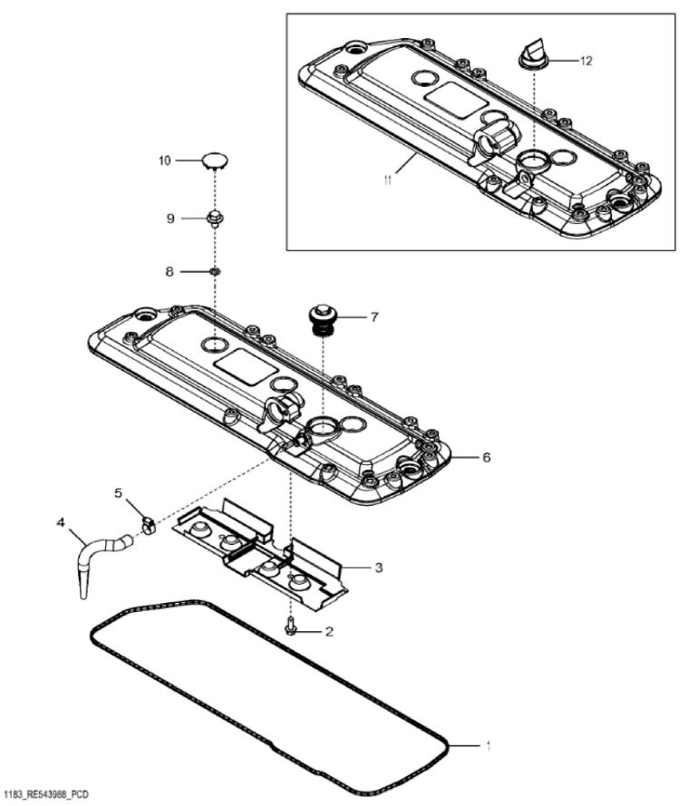
John Deere > Turf And Utility >TRACTOR >6110R - TRACTOR >6110R Tractor (North America Edition, Engine SN: 4045UXXXXXX)(Final Tier 4) >E1 ENGINE 4045HL500-DD22292-ETN122284-ETN122286-ETN131686 >E100 ENGINE 4045HL500-DD22292-ETN122286-ETN131686 4045HL500 >ST400926 - 1183 ROCKER ARM COVER
