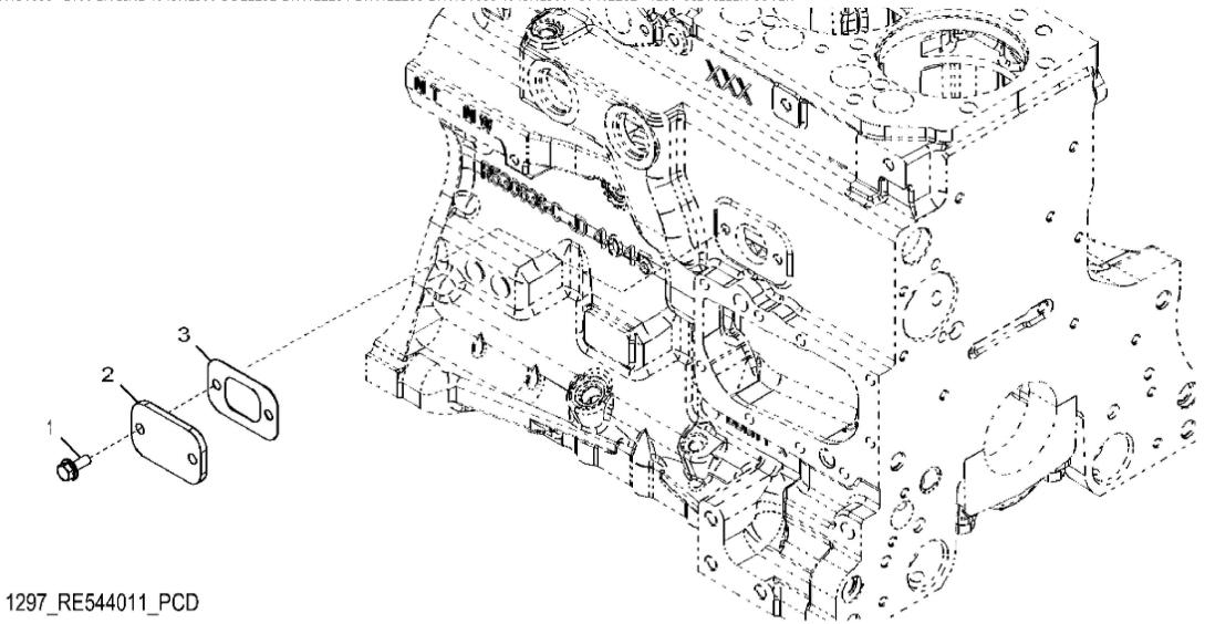
John Deere > Turf And Utility >TRACTOR >6110R - TRACTOR >6110R Tractor (North America Edition, Engine SN: 4045UXXXXXX)(Final Tier 4) >E1 ENGINE 4045HL500-DD22292-ETN122284-ETN122286-ETN131686 >E100 ENGINE 4045HL500-DD22292-ETN122286-ETN131686 4045HL500 >ST402282 - 1297 OIL FILLER COVER
