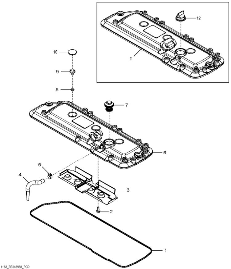
John Deere > Turf And Utility >TRACTOR >6120R - TRACTOR >6120R Tractor (North America Edition, Engine SN: 4045UXXXXXX)(Final Tier 4) >E1 ENGINE 4045HL500-DD22292-ETN122284-ETN122286-ETN131686 >E100 ENGINE 4045HL500-DD22292-ETN122286-ETN131686 4045HL500 >ST400926 - 1183 ROCKER ARM COVER
