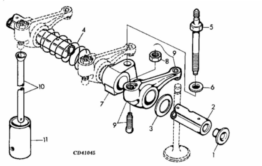
John Deere > Turf And Utility >TRACTOR >5715HC - TRACTOR >5415, 5415H, 5615, 5715 and 5715HC Tractors >20 ENGINE >ST728735 - ROCKER ARM/SHAFT/TAPPET/PUSH ROD
