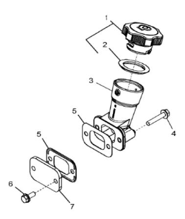
John Deere > Turf And Utility >TRACTOR >5715 - TRACTOR >5415, 5615 and 5715 Tractors (5015 Series) (Worldwide Edition) >20 ENGINE 4045DP057-RE530900 - RE556191 >ST308623 - 1202 OIL FILLER NECK
