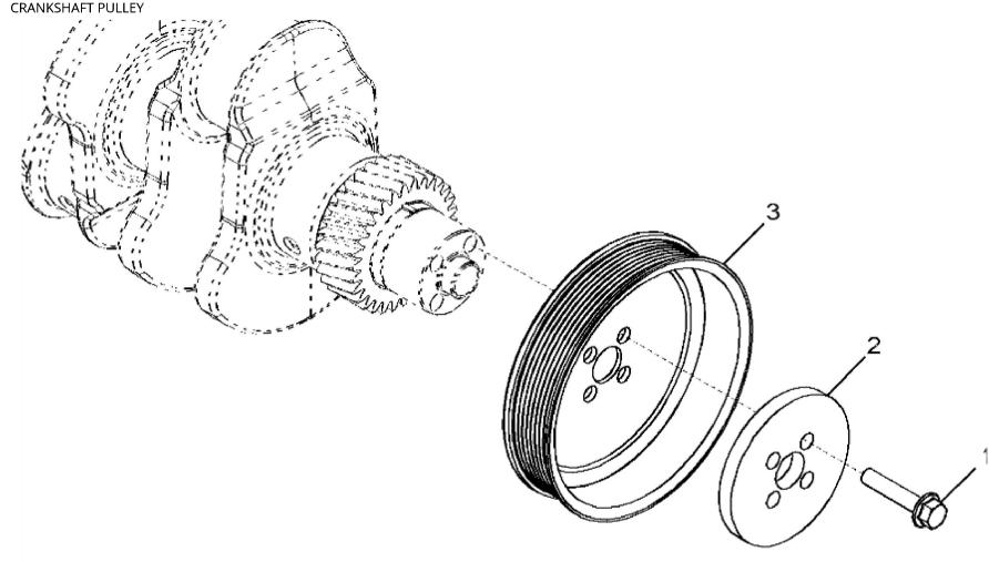
John Deere > Turf And Utility >TRACTOR >5715 - TRACTOR >5415, 5615 and 5715 Tractors (5015 Series) (Worldwide Edition) >20 ENGINE 4045DP057-RE530900 - RE556191 >ST351152 - 1302 CRANKSHAFT PULLEY
