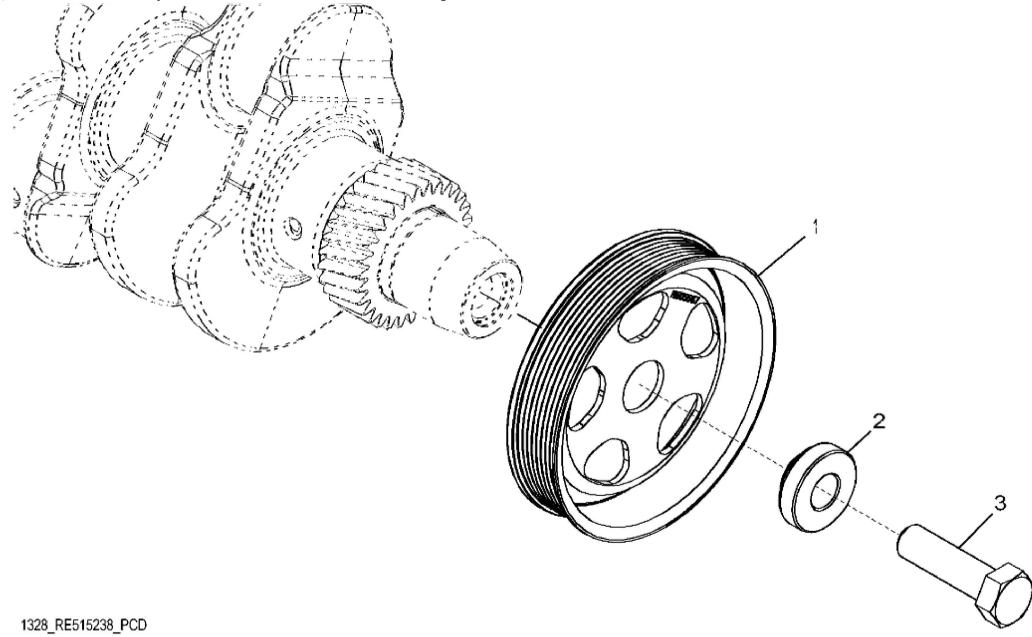
John Deere > Turf And Utility >TRACTOR >5083E - TRACTOR >5083E Tractor (Engine 4045HP058)(Mexico Edition) >20 ENGINE 4045HP058-RE546999 >ST628039 - 1328 CRANKSHAFT PULLEY
