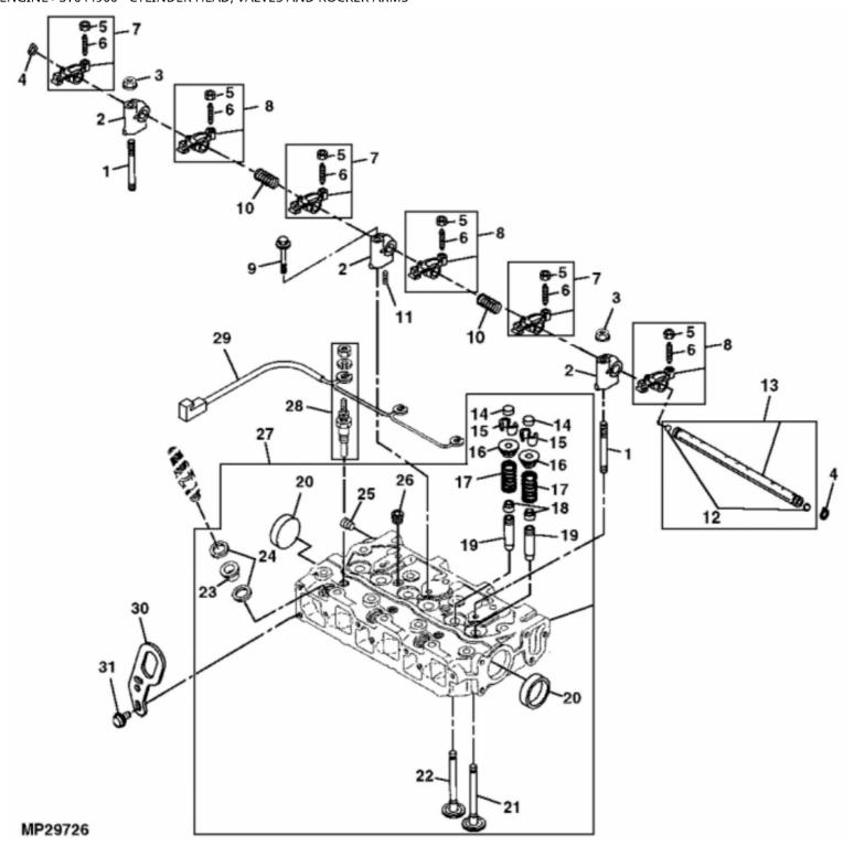
John Deere > Turf And Utility >TRACTOR, COMPACT UTILITY >3TNE74 - TRACTOR, COMPACT UTILITY >2210 Compact Utility Tractor >20 ENGINE >ST644966 - CYLINDER HEAD, VALVES AND ROCKER ARMS
