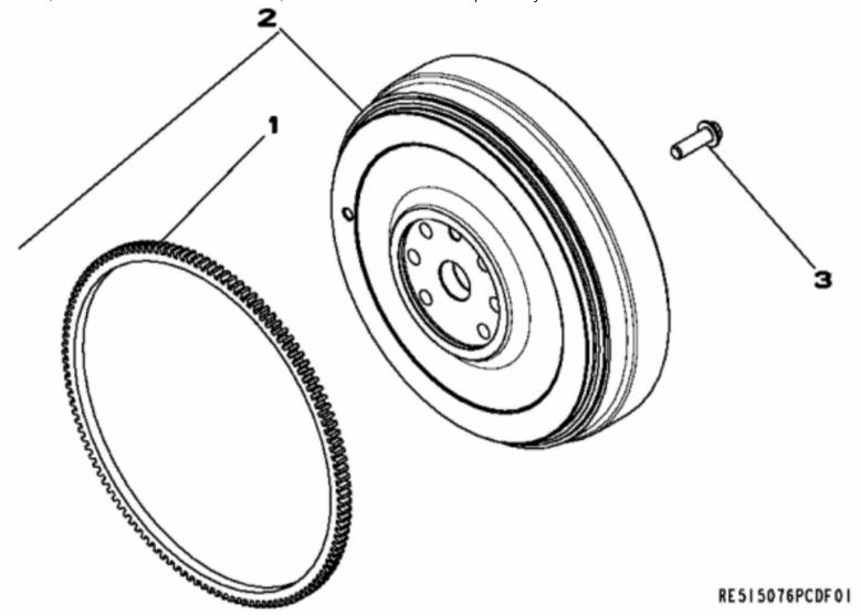
John Deere > Turf And Utility >TRACTOR, COMPACT UTILITY >4120 - TRACTOR, COMPACT UTILITY >4120 Compact Utility Tractor >20 ENGINE 4024TLV04-RE522472 >ST293045 - 1503 FLYWHEEL
