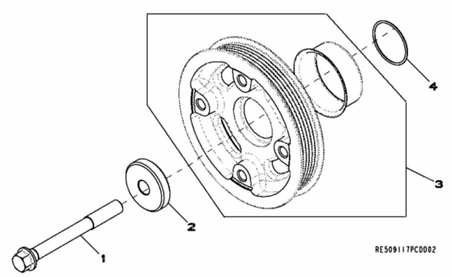
John Deere > Turf And Utility >TRACTOR, COMPACT UTILITY >4120 - TRACTOR, COMPACT UTILITY >4120 Compact Utility Tractor >20 ENGINE 4024TLV04-RE522472 >ST293043 - 1301 CRANKSHAFT PULLEY
