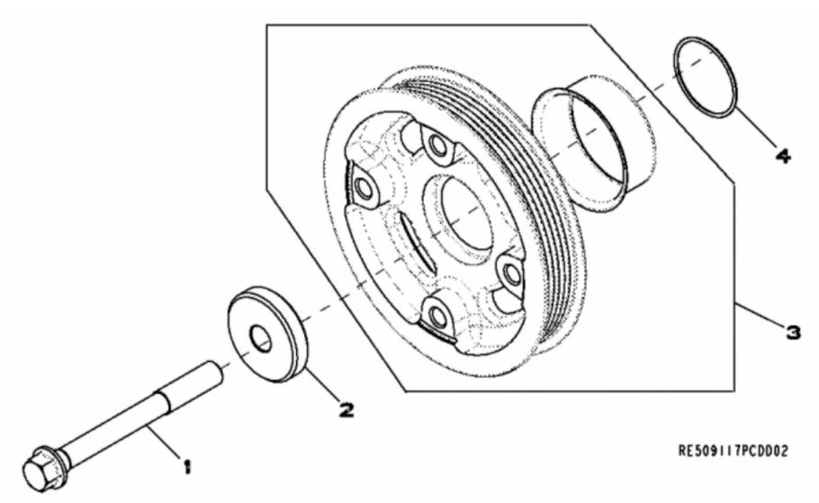
John Deere > Turf And Utility >TRACTOR, COMPACT UTILITY >4720 - TRACTOR, COMPACT UTILITY >4720 Compact Utility Tractor >21 ENGINE 4024TLV03-RE516055 >ST293043 - 1301 CRANKSHAFT PULLEY
