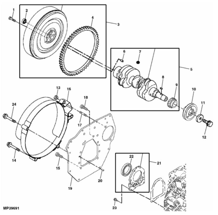
John Deere > Turf And Utility >TRACTOR, COMPACT UTILITY >3TNV76 - TRACTOR, COMPACT UTILITY >2320 Compact Utility Tractor >20 ENGINE >ST149755 - CRANKSHAFT, FLYWHEEL AND MOUNTING FLANGE
