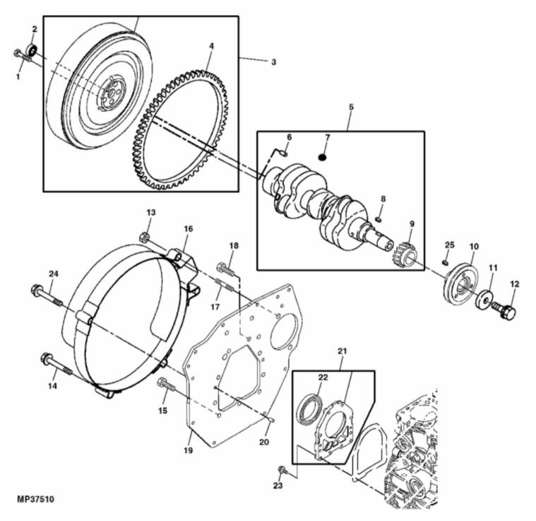
John Deere > Turf And Utility >TRACTOR, COMPACT UTILITY >3TNV76 - TRACTOR, COMPACT UTILITY >2305 Compact Utility Tractor >20 ENGINE >ST150506 - CRANKSHAFT, FLYWHEEL AND MOUNTING FLANGE
