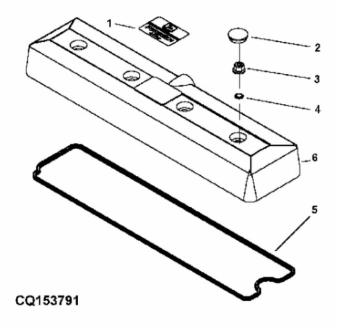
John Deere > Turf And Utility >TRACTOR >5603 - TRACTOR >5603 Tractor (South American Edition) >20 ENGINE >ST357262 - VALVE COVER
