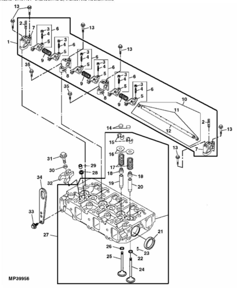
John Deere > Turf And Utility >TRACTOR, COMPACT UTILITY >4105 - TRACTOR, COMPACT UTILITY >4105 Compact Utility Tractor >20 ENGINE >ST151164 - CYLINDER HEAD, VALVES AND ROCKER ARMS
