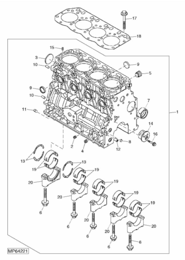
John Deere > Turf And Utility >TRACTOR, COMPACT UTILITY >4TNV88 - TRACTOR, COMPACT UTILITY >4005 Compact Utility Tractor >20 ENGINE >ST150956 - CYLINDER BLOCK AND MAIN BEARINGS
