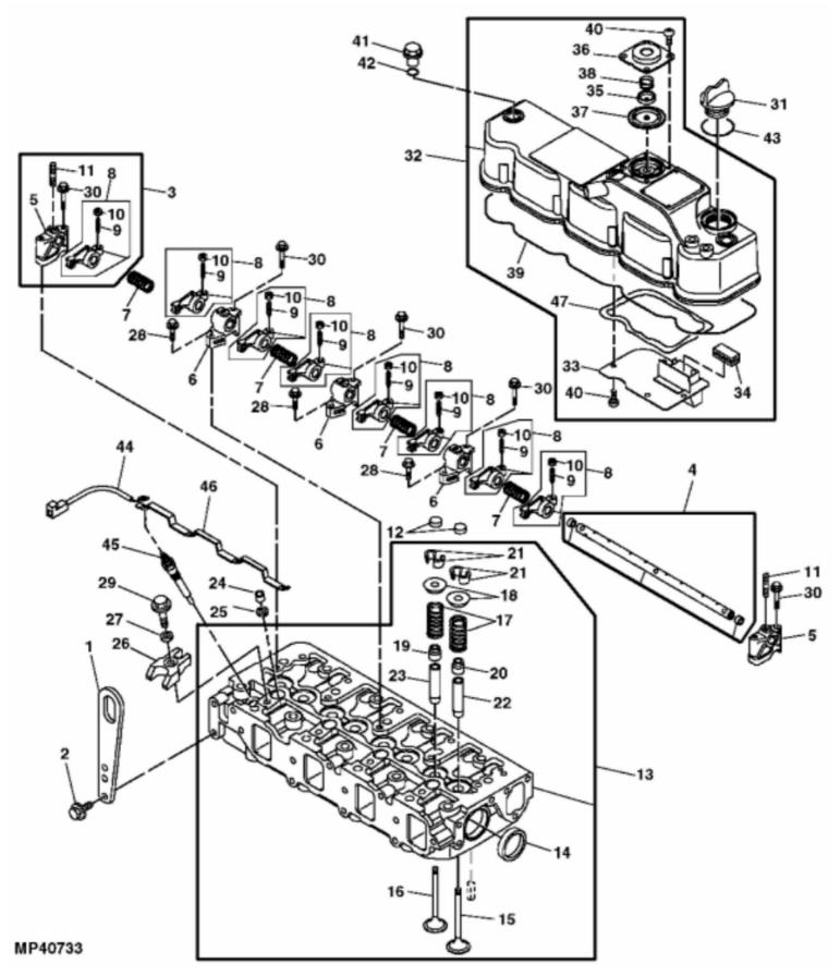
John Deere > Turf And Utility >TRACTOR, COMPACT UTILITY >4TNV88 - TRACTOR, COMPACT UTILITY >4005 Compact Utility Tractor >20 ENGINE >ST150957 - CYLINDER HEAD, VALVES AND ROCKER ARMS
