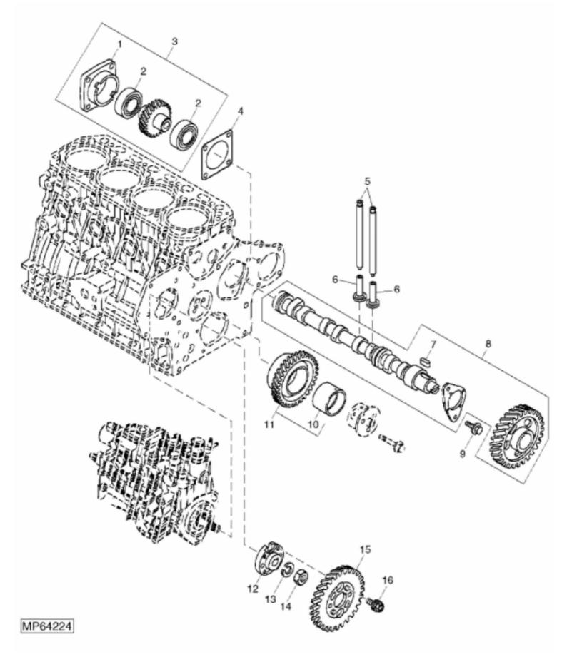
John Deere > Turf And Utility >TRACTOR, COMPACT UTILITY >4TNV88 - TRACTOR, COMPACT UTILITY >4005 Compact Utility Tractor >20 ENGINE >ST150958 - CAMSHAFT AND DRIVING GEARS
