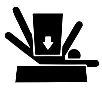
If you must work on a lifted machine or attachment, securely support the machine or attachment.
