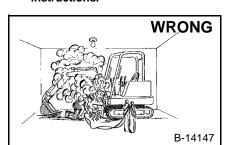
Have good ventilation when welding or grinding painted
