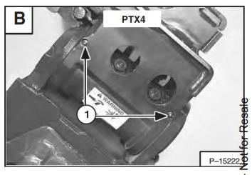
Apply the grease until clean grease flows from the grease relief valves (Item 1) [C] & [D].
