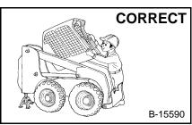
Use the correct procedure to lift or lower operator cab.
