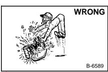
Lead-acid batteries produce flammable and explosive gases.
