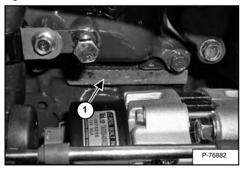
The engine serial number is located on the side of the engine (Item 1) [Figure 2] above the alternator.
