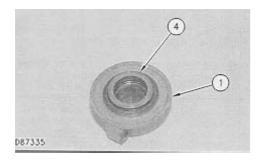
**NOTE:** If the Duo-Cone Seals are to be used again, put identification marks on the seals to assure that they are assembled and installed in their original positions.
