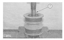
7. Use a press and roller shaft (7) to remove the bushing assembly on the opposite side.
