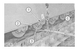
**4.** Fasten a hoist and suitable lifting device to Tool (C). Put Tool (C) in position under the roller as shown.
