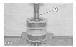
8. Rotate the roller assembly over 180 degrees. Use a press and roller shaft (7) to remove the remaining bushing assembly.
