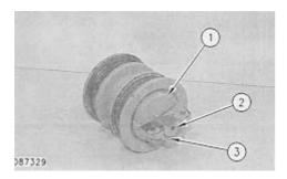
**1.** Use a hammer and punch, to remove the plug out of stopper (2).
