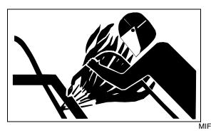
Flammable spray can be generated by heating near pressurized fluid lines, resulting in severe burns to yourself and bystanders. Do not heat by welding, soldering, or using a torch near pressurized fluid lines or other flammable materials. Pressurized lines can be accidentally cut when heat goes beyond the immediate flame area.
