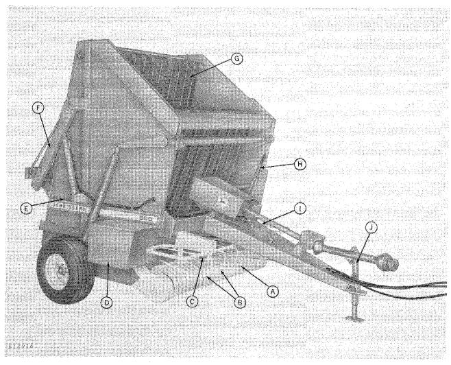
A—Pickup B—Compressors C—Twine Tube
