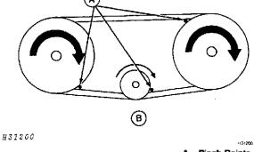
A—Pinch Points B—Belt Drive Keep guards and shields in place at all times while operating the combine. Always disengage separator and shut off engine before removing guards or shields.
