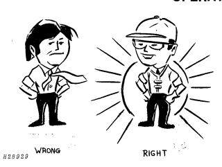
Clothing worn by operator must be fairly tight and belted. Loose jackets, shirts, or sleeves must never be worn.
