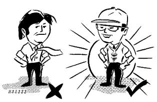
Clothing worn by operator must be fairly tight and belted. Loose jackets, shirts, or sleeves must never be worn.
