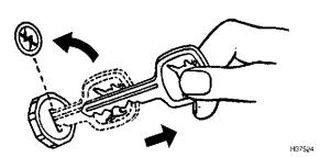
Before leaving combine unattended, turn off engine and remove keys. Support header with hydraulic cylinder safety stop if it is necessary to go under the header or feeder house. See the combine Operator's Manual for complete safety information.
