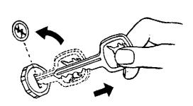
Before leaving the combine unattended, turn off engine and remove keys, support the header with either the hydraulic cylinder safety stop, or lower it to the ground. The gearshift lever must be in neutral and the parking brake engaged.
