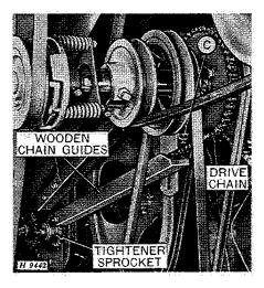
After completing drive belt adjustments, check the drive chain tension. The drive chain should be just tight enough to run without climbing or jumping sprockets. Adjust, as necessary, with tightener sprocket and adjust wooden chain guides so they are directly under the chain, with a slight clearance between chain and ends of guides. Adjust chain guide front support "C" so chain is centered in guides.
