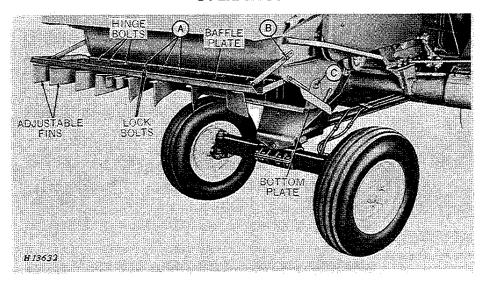
The straw chopper chops the straw into short lengths and, at the same time, bruises it so that decomposition can take place rapidly. The adjustable fins can be adjusted to spread the material in an even, thin layer over a wide area behind the combine. They also can be adjusted to keep the material off the uncut crop.
