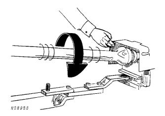
Keep guards and shields in place at all times while operating the combine. Always disengage tractor PTO and shut off engine before removing guards or shields.
