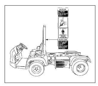
To avoid injury from crushing always wear seat belt. Do not jump from machine.
