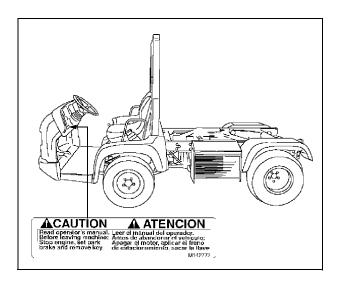
Read operator's manual. Before leaving machine: Stop engine, set park brake and remove key.
