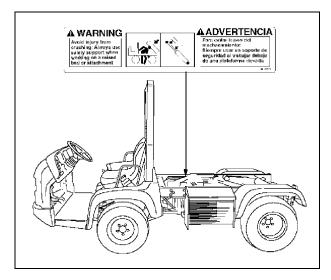
Picture Note: Labels are located on each vehicle frame side rail.
