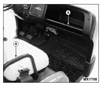
Hand holds (A) are provided for operator and passenger balance when driving over rough terrain. Use dash bar and side rails on seats for stability.
