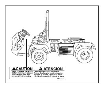
Read operator's manual. Before leaving machine: Stop engine, set park brake and remove key.
