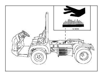
Picture Note: "HOT" muffler warning stamped into the top of the vehicle muffler.
