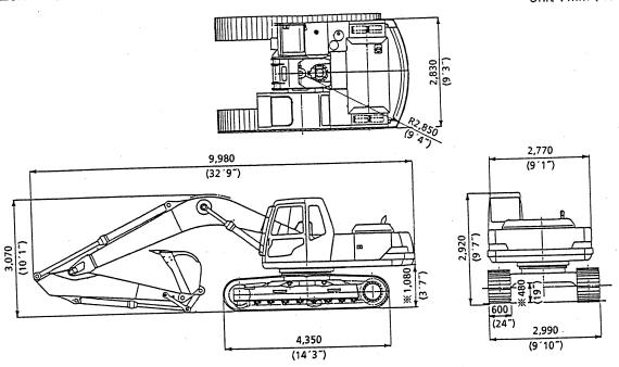
■ SK220Lc ( 6.02m (19ft 9in) BOOM + 2.98m (9ft 9in) ARM-ATTACHED STANDARD MACHINE )
