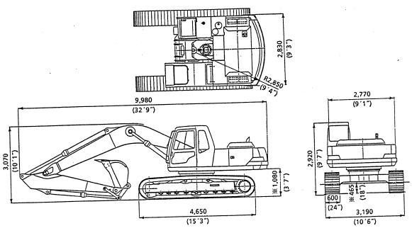
lacksquare The figures marked lacksquare in the illustration do not include the shoe embossment (26mm) ( 1.02" ) .
