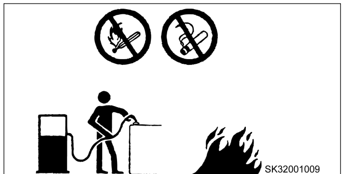
KEEP FIRE AWAY FROM FUEL & OIL
