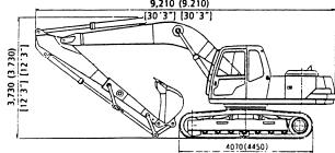
SK200 (WITH 5.6m (18ft 4in) BOOM + 2.94m (9ft 8in) ARM + 1.5m (4ft 11in) EXTENSION ARM )
