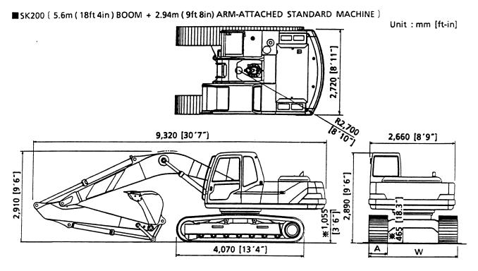
SK200LC ( 5.6m ( 18ft 4in ) BOOM + 2.94m ( 9ft 8in) ARM-ÅTTACHED STANDARD MACHINE )
