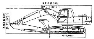
SK200 (WITH 5.6m (18ft 4in) BOOM + 2.4m (7ft 10in) ARM + 1.5m (4ft 11in) EXTENSION ARM )
