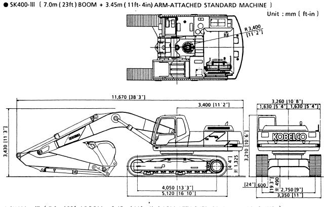
• SK400LC-III (7.0m (23ft) BOOM + 3.45m (11ft-4in) ARM-ATTACHED STANDARD MACHINE
