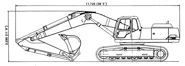
• SK400-III, SK400Lc-III ( WITH 7.0m (23ft ) BOOM + 4.9m (16ft 1in) ARM )
