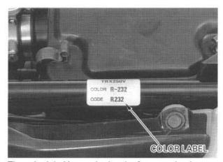
The color label is attached to the frame under the seat as shown. When ordering color-coded parts, always specify the designated color code.
