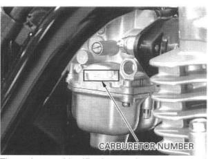
The carburetor identification numbers are stamped on the right side of the carburetor body as shown.
