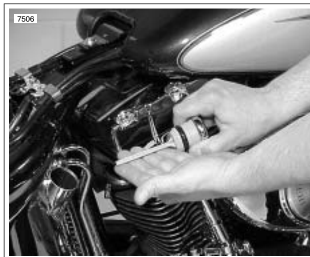
Figure 1-1. Checking Oil Tank Level
